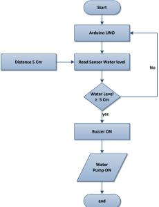
Figure 3. The working principle of the tool
