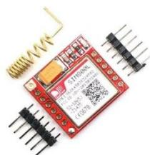
Gambar 2. Modul GSM/ GPRS SIM 800L
