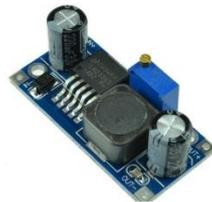
Gambar 3. Converter Step Down Power Supply Modul
