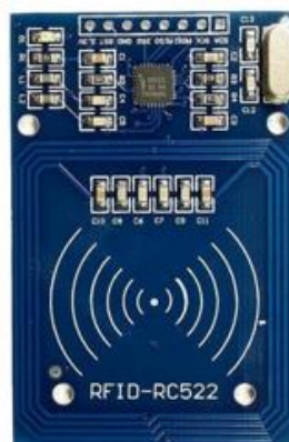
Gambar 2. RFID Reader tipe RC522
