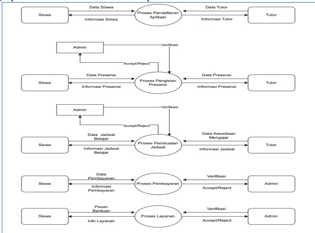
Gambar-4. Data Flow Diagram level 1
