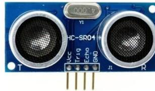
Gambar 2. Sensor Ultrasonik HC-SR04
