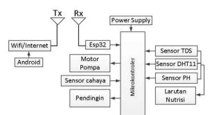
Figure 4. Overall Block Diagram (Hardware)
