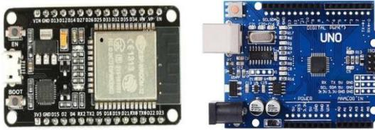
Figure 2. Arduino Uno and Module of ESP 32
