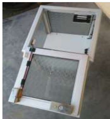
Figure 9 Use of Doorlock and Magneticlock in Charity Box Security Systems
