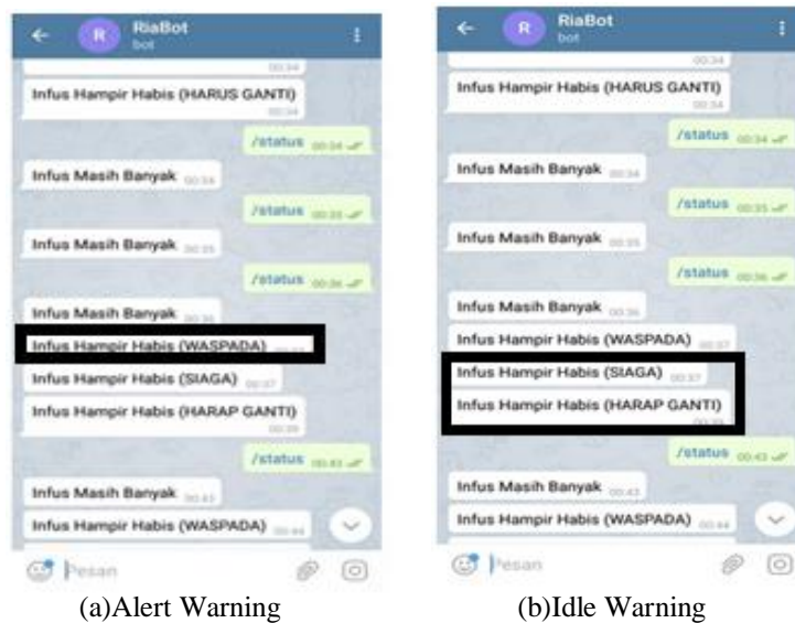
Figure 7.(a) and (b) Notification Via Telegram
