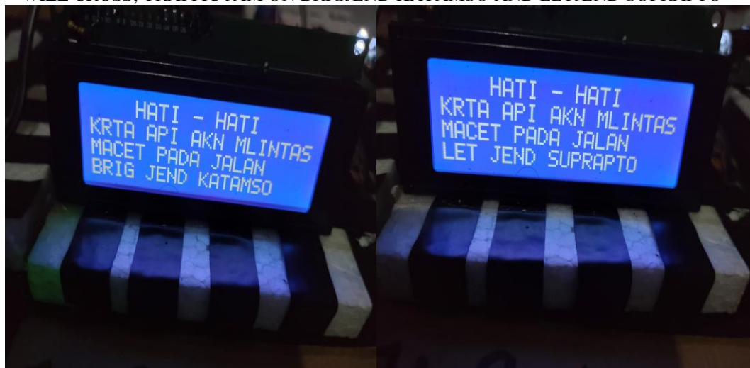
Fig. 13. LCD Display Process when the traffic congestion occurs at Brigjen Katamso and Letjen Suprpto
