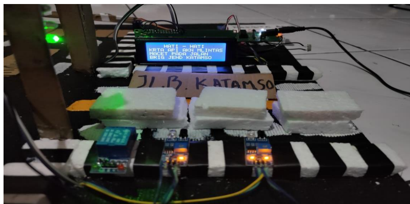
Fig. 7. IR_Photodiada Sensor State Process Detects Congestion Long On Jalan Brigadier General Katamso
