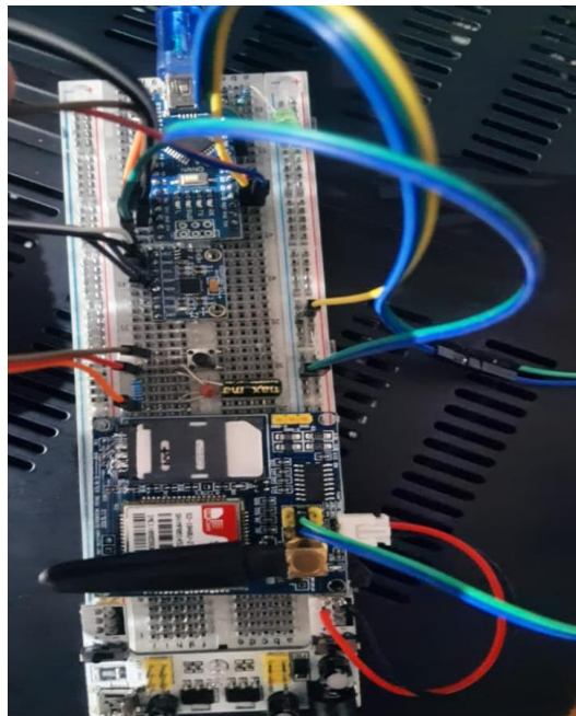
Figure. 4 Motion sensor detection prototype with MPU6050 Source : researcher property
