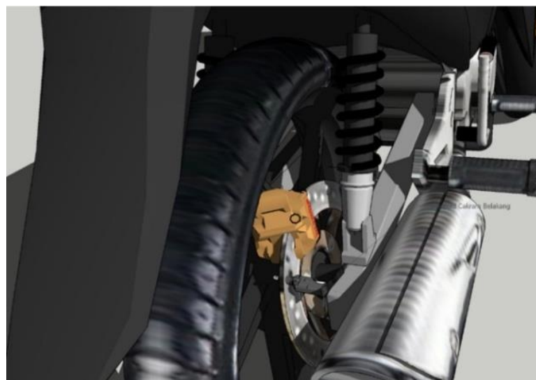
Figure 9 Automatic Double Lock Illustration on Rear Discs
