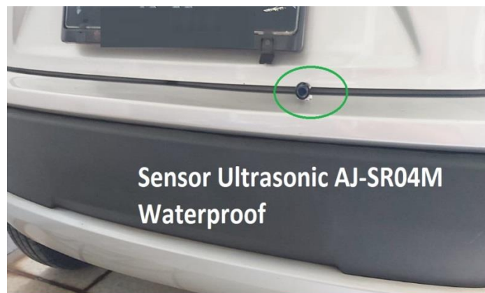
Fig 5 Application of parking sensors on vehicles Source: Researcher Property
