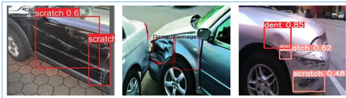
Figure 3, Detection results using YOLO for bonnets, doors, and bumper. Source: Researcher property
