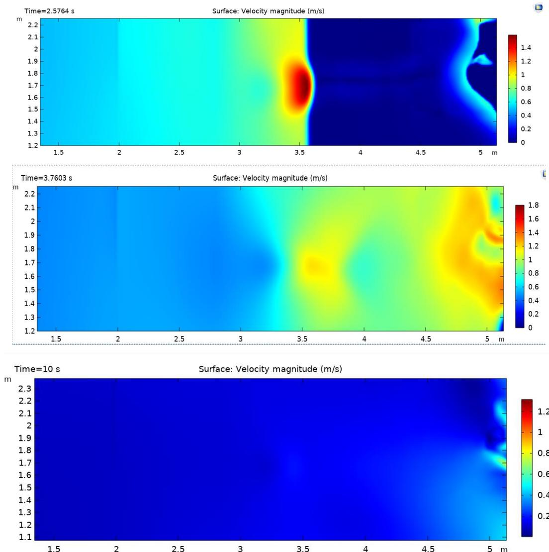
**Figure 3.** Simulation of the breaking speed of the wave  $t = [0,10]$
