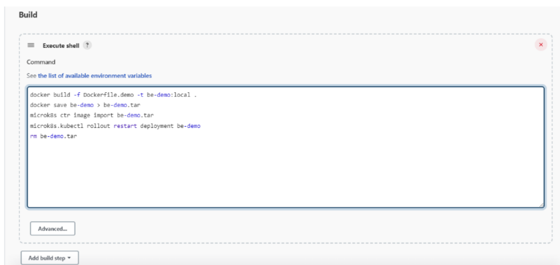
Fig 10. Build Command Configuration
