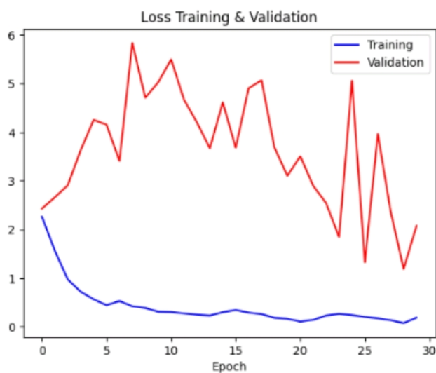
Fig. 4. Graph of Loss Training and Validation on Inception V3 Model
