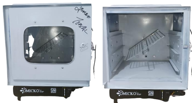
Figure 5 Automatic steak griller (Source:Researcher Property)
