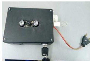
Fig. 5 The overall motorcycle security system appears using raspberry pi3
