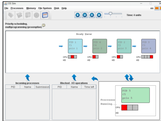
Fig 6. C5 is executed at 4 ms.
