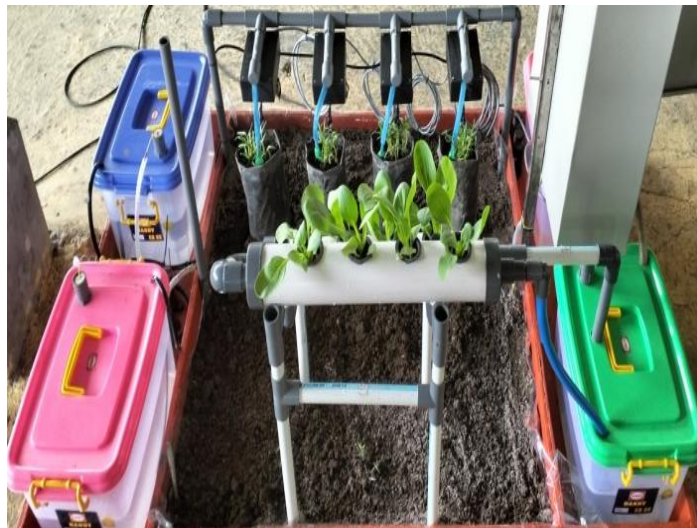
Fig. 4 Embedded Smart Farming Prototype for Soil and Hydroponic Planting Media (side view).
