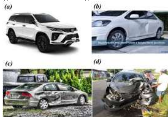
Fig. 2 Representative samples of vehicle damage severity categories: (a) Normal, (b) Light, (c) Medium, (d) Heavy.
