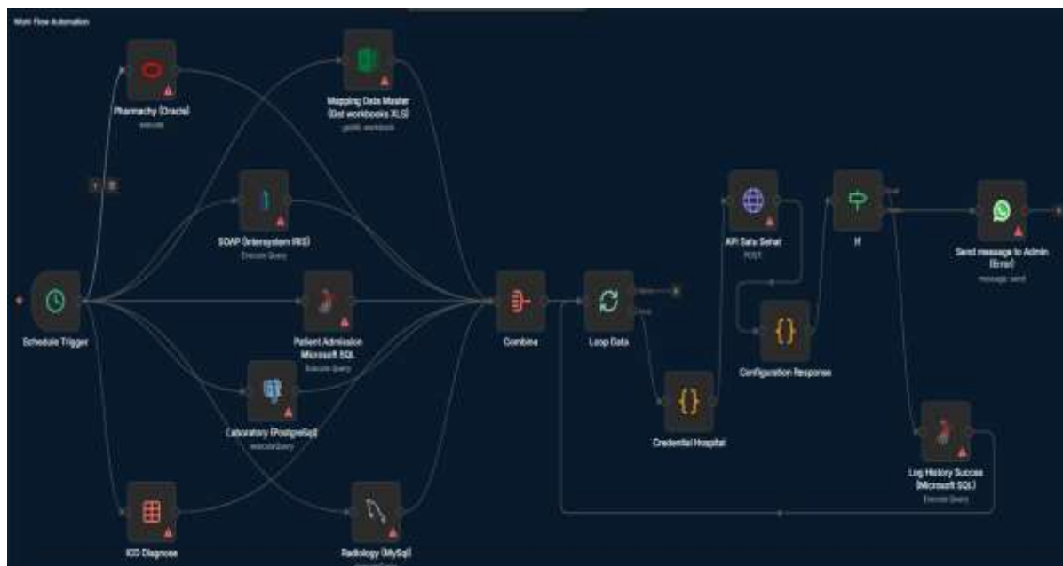
Fig. 3 Automated n8n Workflow for SATUSEHAT Integration
