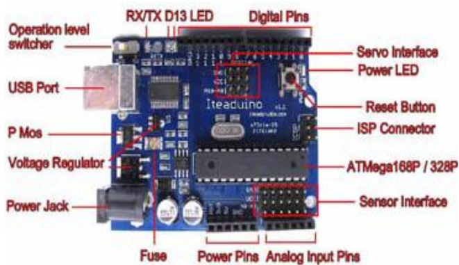
Gambar 1 Tampilan Board Arduino Uno
